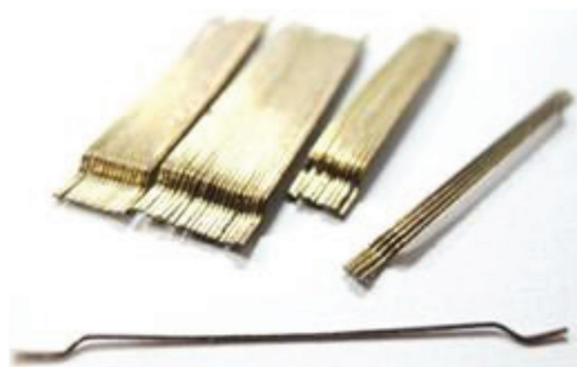
Fig. 2—Presence of hooked-end steel fibers.
