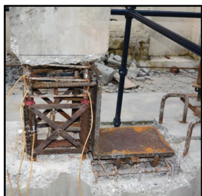
(a) Base plate connection with the coupler-box assembly at column base
