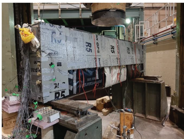
Fig. 6—Power-blankets wrapped on shear beam for heating before start of test.
