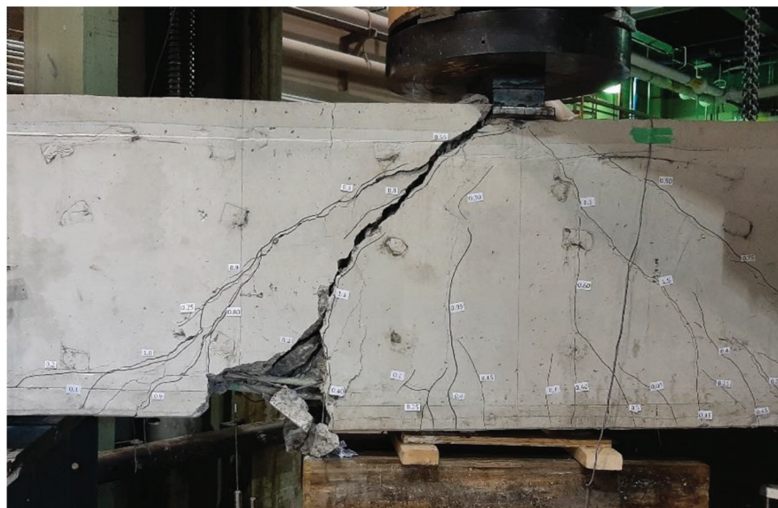
Fig. 10—Control beam failure and stirrup rupture (north face of beam).
