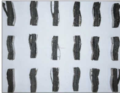
Severely damaged exterior grid links
