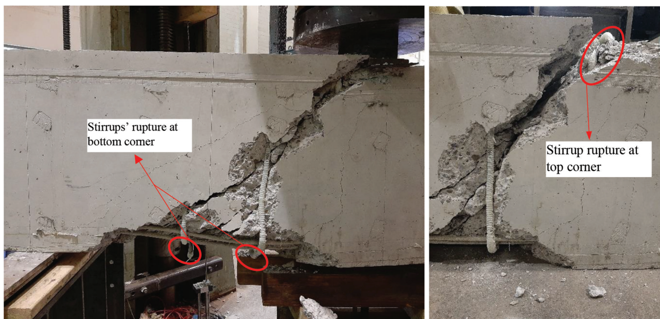
Fig. 15—Failure of Beam 2 (shear-critical conditioned beam)-south face of beam.
