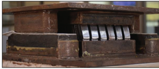
Damaged damper with yielded links
