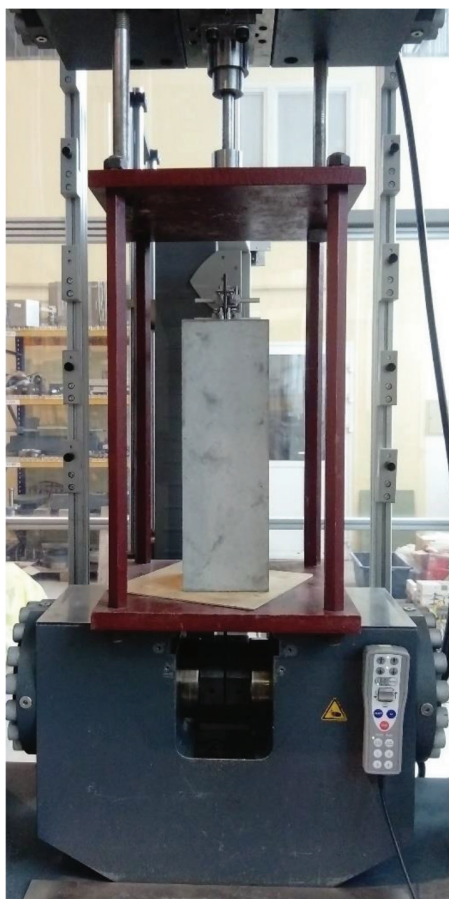
Fig. 3—General view of concrete specimen during testing.
