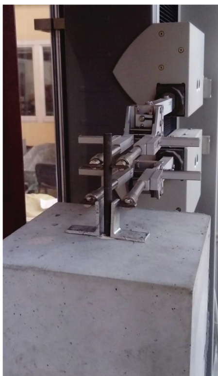
Fig. 4—Extensometer mounted at free end of plain steel prestressing wire of 7 mm during testing.
