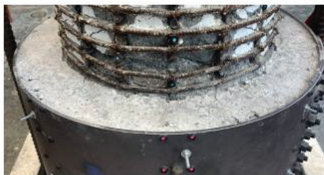
Fig. 15—Damage comparison after Repair No. 4 test with loose grout removed on: (left) north; and (right) south sides.
