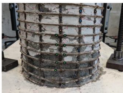
Fig. 7—Damage conditions of: (a) Repair No. 1; (b) Repair No. 2; and (c) original plastic hinge of Repair No. 1 prior to repair.
