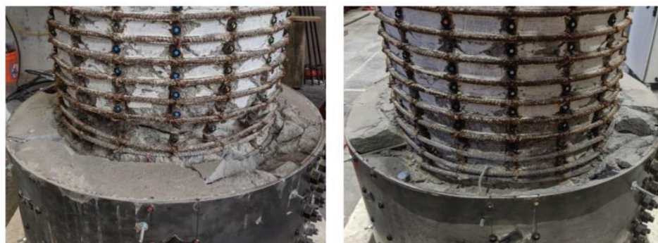
Fig. 12—Damage comparison of: (left) north; and (right) south sides after Repair No. 3 test with loose grout removed.
