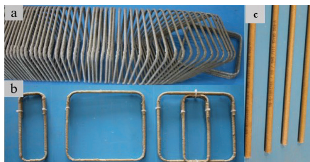
Fig. 1—(a) GFRP continuous square spiral stirrups; (b) GFRP individual square tie stirrups; and (c) GFRP bars.
