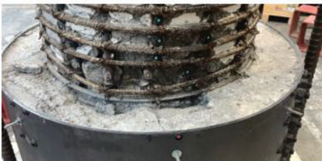
Fig. 15—Damage comparison after Repair No. 4 test with loose grout removed on: (left) north; and (right) south sides.
