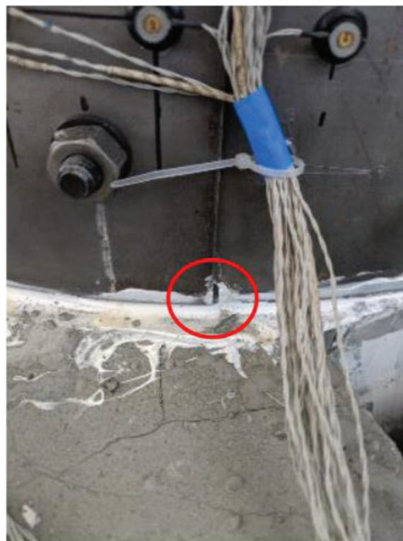
Fig. 9—Ruptured silicone seal of Repair No. 1.
