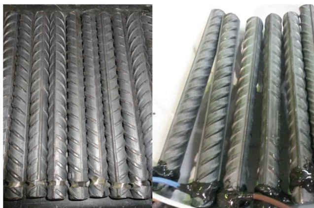
Fig. 1—Carbon steel reinforcing bars glued to copper wires for electrical connection.
