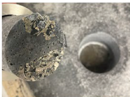
Fig. 10—Post-test of cementitious core samples after pulloff testing, showing fracture surface: (a) pulloff testing; and (b) interface failures.
