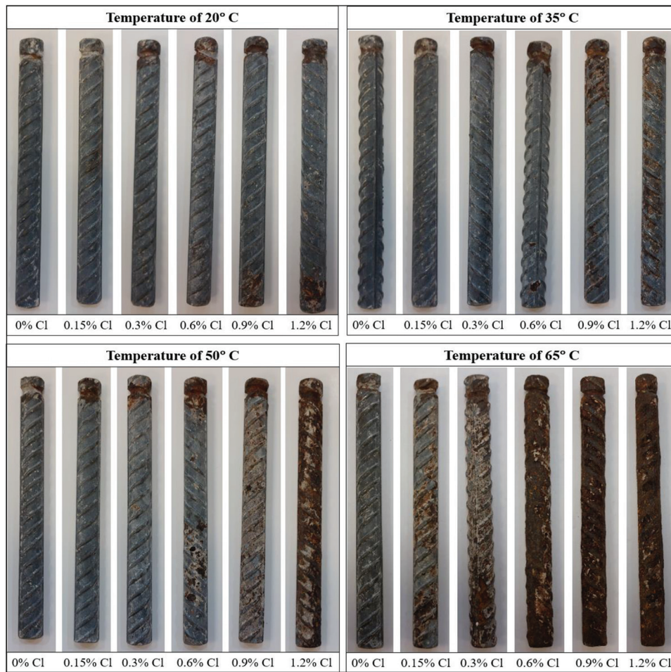
Fig. 9—Photos of reinforcing bars exposed to different temperatures and chloride contents (Source B).
