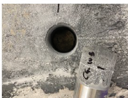
Fig. 9—Post-test of epoxy core samples after pulloff testing, showing fracture surface: (a) no failure observed; and (b) interface failure.
