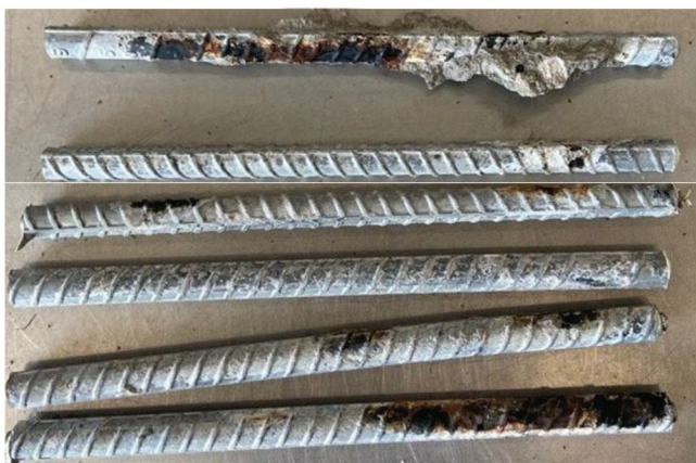
Fig. 12—SE test: specimen A1094-4 after 96 weeks of testing. Top mat (top) and bottom mat (bottom).
