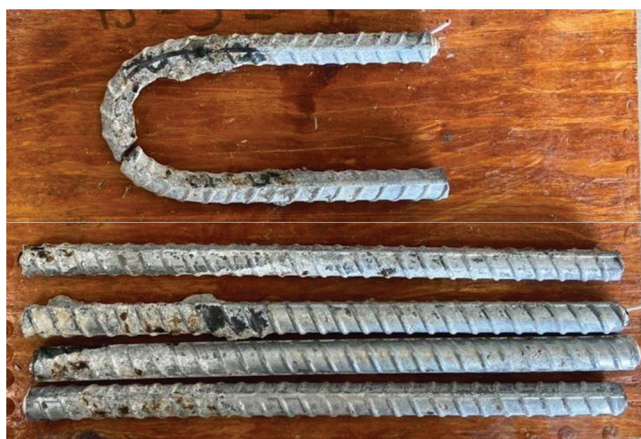
Fig. 15—SE test: specimen A1094-b-2 after 96 weeks of testing. Top mat (top) and bottom mat (bottom).
