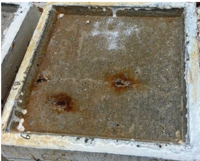
Fig. 17—SE test: surface staining on specimen with conventional reinforcement.
