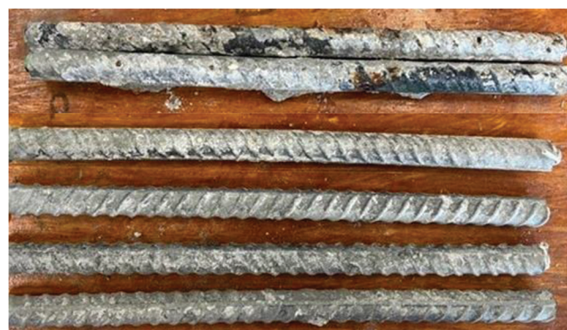
Fig. 9—SE test: specimen A767-3 after 96 weeks of testing. Top mat (top) and bottom mat (bottom).
