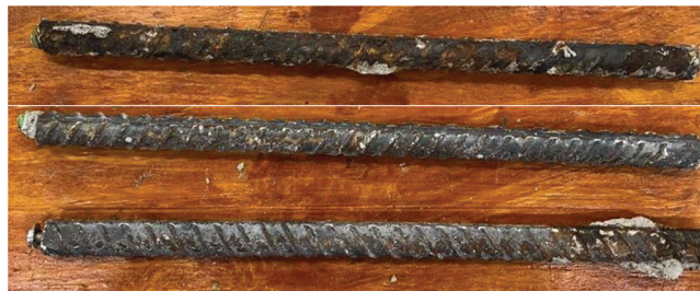
Fig. 18—CB test: specimen Conv-I-1 after 96 weeks of testing. Top mat (top) and bottom mat (bottom).
