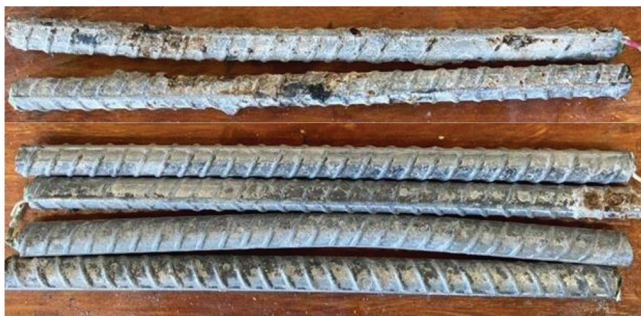
Fig. 10—SE test: specimen A767-2 after 96 weeks of testing. Top mat (top) and bottom mat (bottom).
