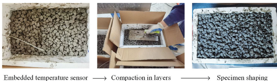
Fig. 1—Test piece fabrication process.
