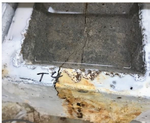
Fig. 8—CB test: cracking of concrete in specimen Conv-I-3.
