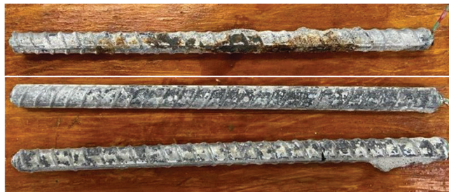
Fig. 13—CB test: specimen A1094-6 after 96 weeks of testing. Top mat (top) and bottom mat (bottom).
