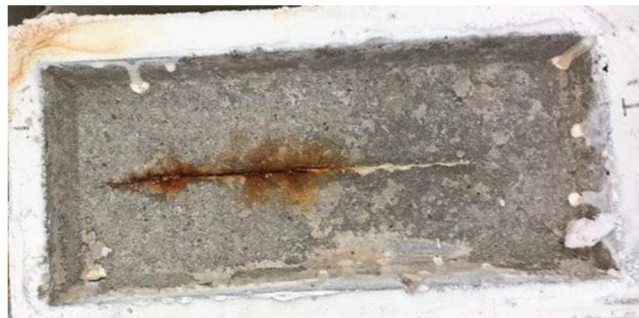
Fig. 19—CB test: surface staining on specimen with conventional reinforcement.
