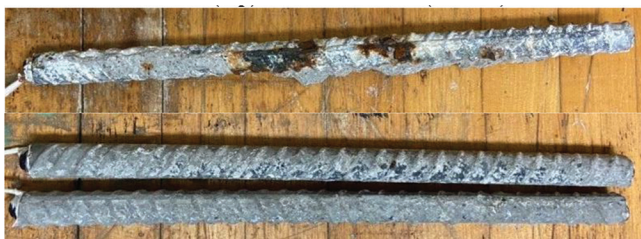
Fig. 11—CB test: specimen A767-3 after 96 weeks of testing. Top mat (top) and bottom mat (bottom).
