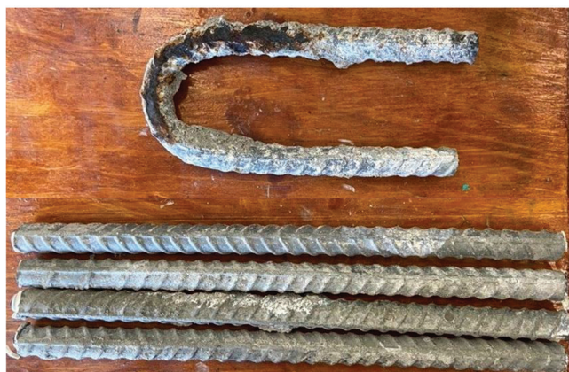
Fig. 14—SE test: specimen A767-b-2 after 96 weeks of testing. Top mat (top) and bottom mat (bottom).
