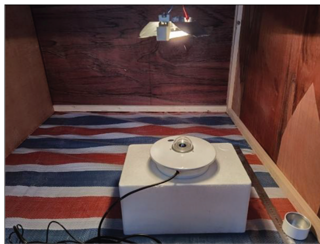
Fig. 2—Indoor heat source: tungsten iodine lamp.
