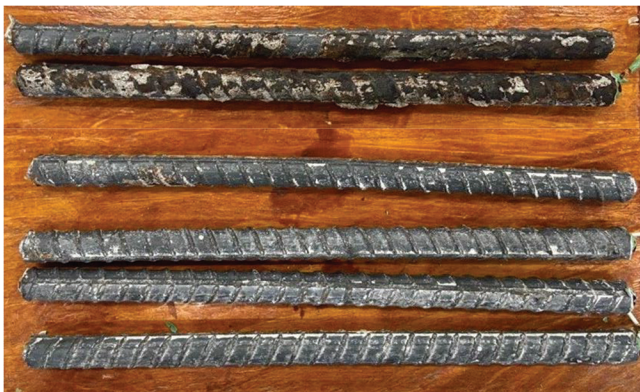
Fig. 16—SE test: specimen Conv-II-1 after 96 weeks of testing. Top mat (top) and bottom mat (bottom).
