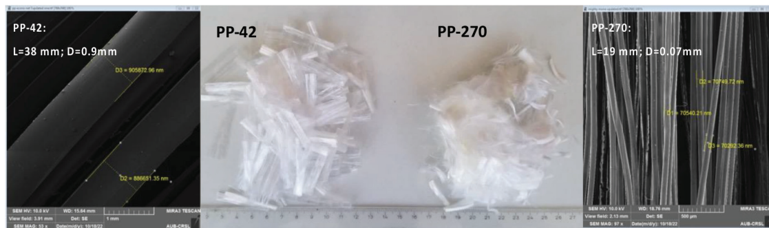
Fig. 1—Photos and SEM images for PP-42 and PP-270 fibers (Al Ghali et al. 2023).
