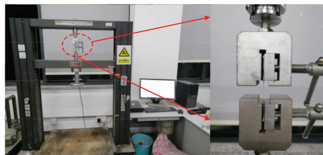
Fig. 3—Universal testing machine for quasi-static tensile test.
