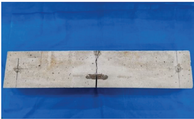
Fig. 13—Mode-I fatigue fracture for specimen C20-0.9.
