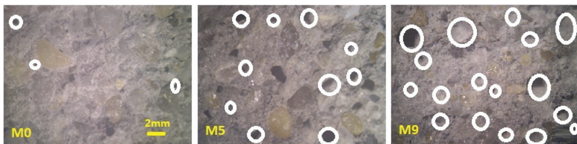
Fig. 5—Porosity analysis of samples by binocular microscope. White circles indicate air voids formed in mortar matrix due to inclusion of AEA.
