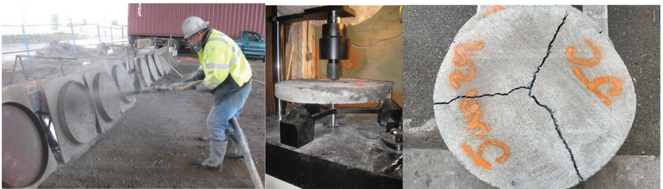
Fig. 10—Shooting and production of RDP (left); testing (middle); and failure pattern (right).
