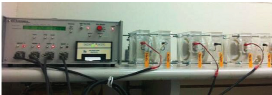
Fig. 1—RCPT testing setup.
