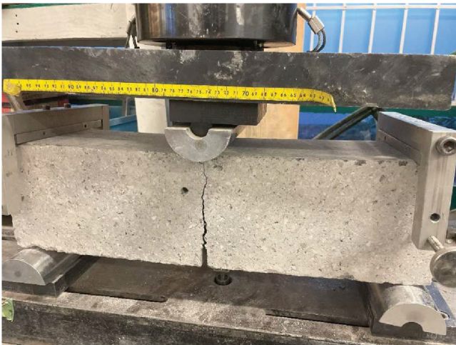
Fig. 5—Fiber-reinforced wet-mix shotcrete notched beam tested according to EN 14651.
