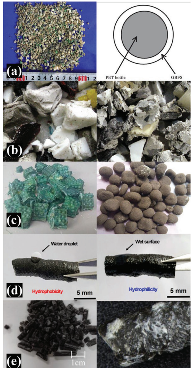
Fig. 2—Surface coating methods for plastic aggregate with different coating materials: (a) blast-furnace slag powder 36 ; (b) cement paste 37 ; (c) volcanic sand 46 ; (d) acrylic-based resin 48 ; and (e) silicone amine resin. 51
