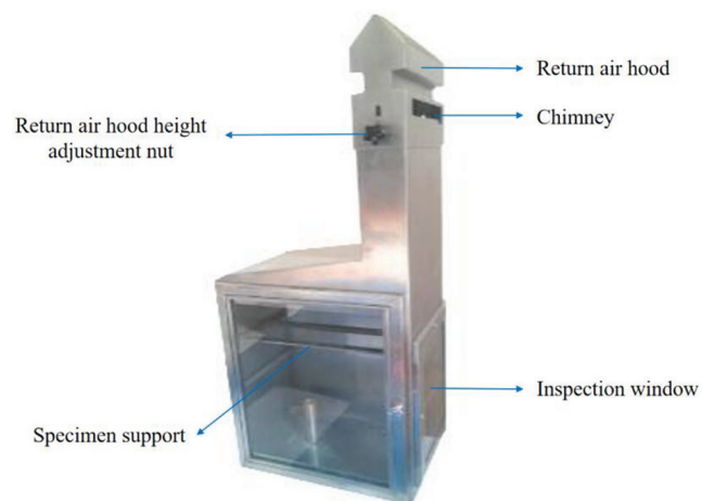
Fig. 3—Tunnel fireproof mortar combustion test machine.
