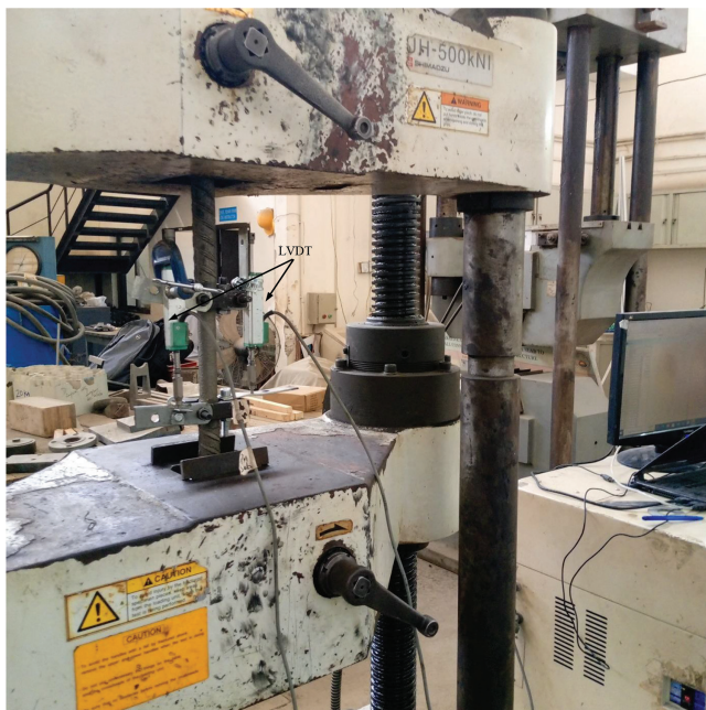
Fig. 4—Tensile strength testing of reinforcing bar.
