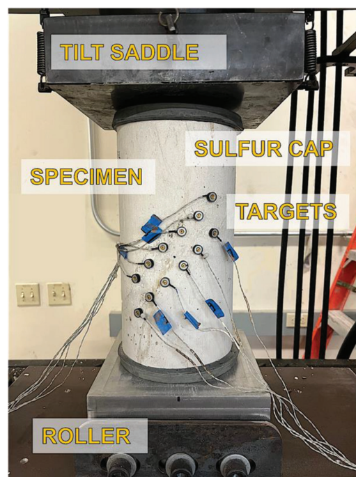
Fig. 2—Test setup of slant shear test.
