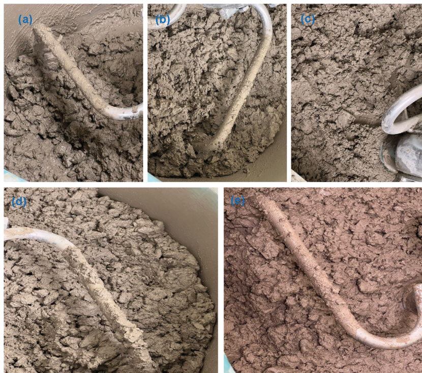
Fig. 4—Images captured from different mixtures after completion of mixing process: (a) control mixture; (b) optimized control mixture; (c) 0.37 w/c mixture; (d) 5% low-cement mixture; and (e) 10% low-cement mixture.
